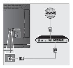
Connect the output of external modem to »LAN« socket with Cat 5 cable.
